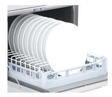
Partial double skin undercounter dishwasher with deep drawn rack guides (patent pending) with a height of 82 cm and door opening of 36.5 cm for washing of up to 32.5 cm high objects. Dual flow pump and full double skin door promote particularly silent operation. Standard equipment includes **ProStrain** integral shock-proof composite material tank filter and double filter on pump intake.
